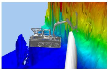
Figure 14: Illustration from Scanmudring Monitoring system, based on survey, post rock breaker operation. Scanmachine with drilling equipment.
