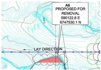
Figure 18: Illustration from "S.o:W for outcrops removal close to Pre-Lay IW12", describing the outcrop east of Holmengraa lighthouse.
