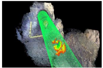
Figure 15: Intermediate Photogrammetry outside the tunnel exit, color codes revealing remaining rock to be removed. The tunnel extension/planned pipeline route is indicated with the green mesh.
