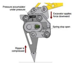
Figure 2: Illustration showing hydraulic ripper used for the project.
