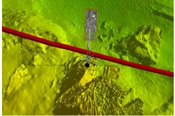
Figure 16: Illustration from Scanmudring Monitoring system, based on survey from the pipe lay route. Planned angle of attack for breaking off the outcrop tip west of Holmengraa lighthouse.
