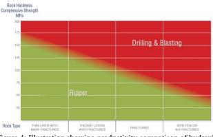
Figure 4: Illustration showing productivity comparison of hydraulic ripper and blasting. Chart from supplier of hydraulic ripper.
