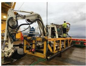
Figure 1: Picture showing Scanmachine#3, in this case placed in basket, equipped with the ripper tooth.
