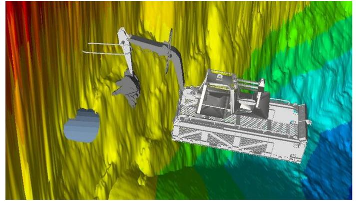
Figure 13: Illustration from Scanmudring Monitoring system, based on rock face as found survey. Scanmachine with rock breaker equipment.
