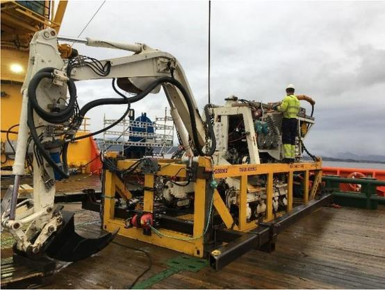
Figure 1: Picture showing Scanmachine#3, in this case placed in basket, equipped with the ripper tooth.
