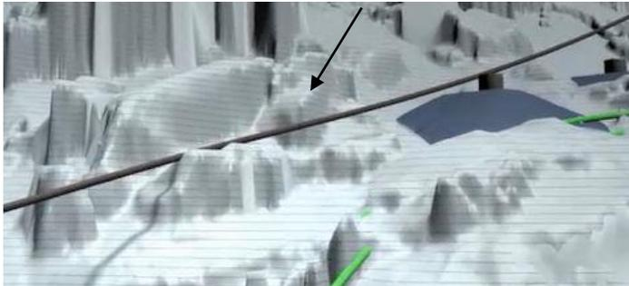
Figure 19: Illustration showing simulation of pipe lay, with terrain based on survey from the pipe lay route. The arrow points out the area of concern, east of Holmengraa lighthouse, at 495meters water depth.
