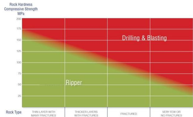
Figure 4: Illustration showing productivity comparison of hydraulic ripper and blasting. Chart from supplier of hydraulic ripper.
