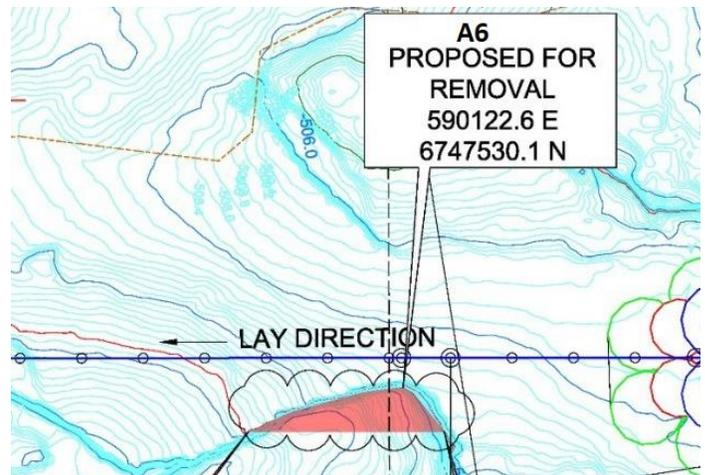
Figure 18: Illustration from "S.o:W for outcrops removal close to Pre-Lay IW12", describing the outcrop east of Holmengraa lighthouse.
