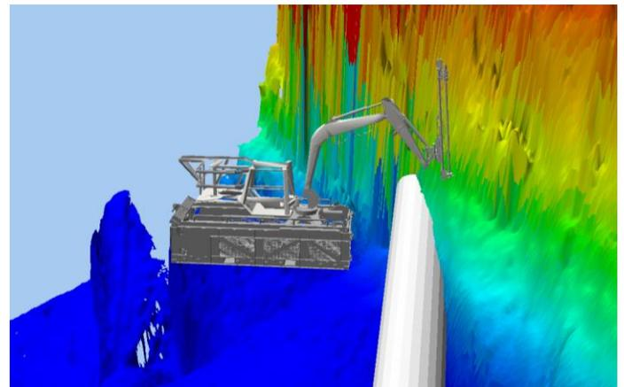
Figure 14: Illustration from Scanmudring Monitoring system, based on survey, post rock breaker operation. Scanmachine with drilling equipment.
