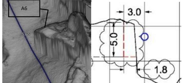
Figure 17: Illustrations from "SOW: For outcrops removal close to Pre-Lay IW12", and 3D graphic from Equinor ST17527-report, describing the outcrop east of Holmengraa lighthouse.
