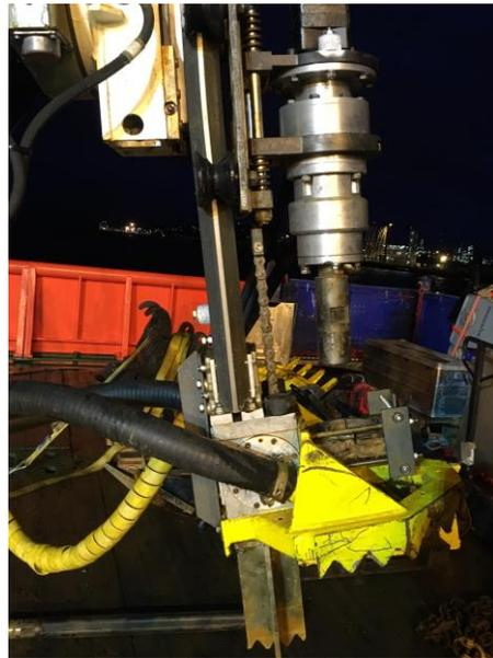
Figure 6: Picture showing rotary head and base of drill rig.
