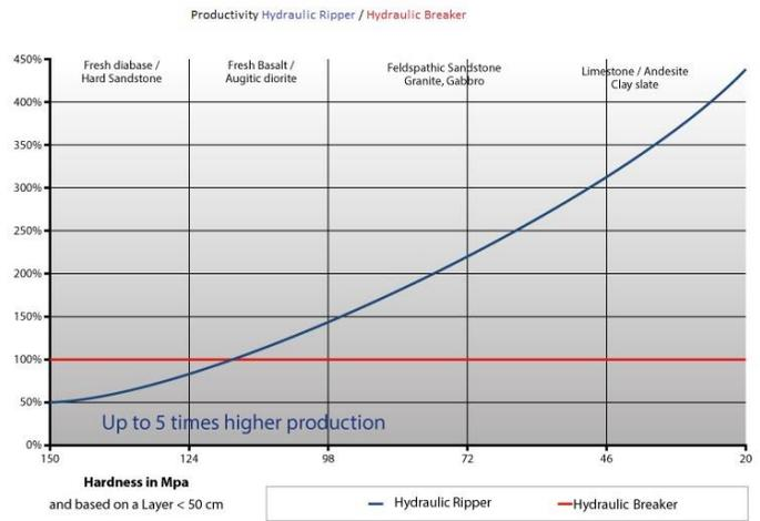
Figure 3: Illustration showing productivity comparison of hydraulic ripper and hydraulic breaker. Chart from supplier of hydraulic ripper.
