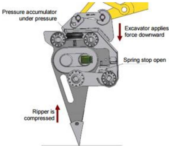
Figure 2: Illustration showing hydraulic ripper used for the project.
