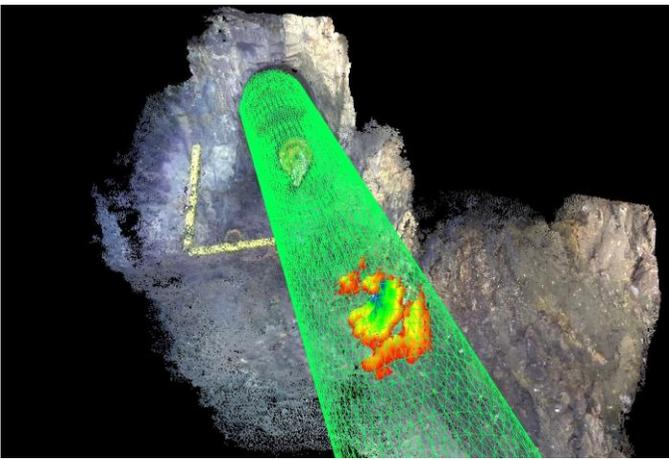
Figure 15: Intermediate Photogrammetry outside the tunnel exit, color codes revealing remaining rock to be removed. The tunnel extension/planned pipeline route is indicated with the green mesh.
